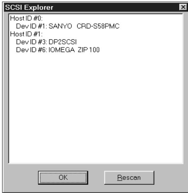
The SCSI Explorer identifies all the SCSI cards and devices installed on your system. Each card is identified by a unique HostID. If devices are attached to a SCSI card, they will be shown by a DevID.
