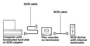
Place the device with the internal terminator at the end of the chain and do not add any additional terminators. If any other external device has an internal terminator, the terminator will have to be removed according to the manufacturer's directions.
