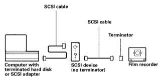
Place a terminator between the SCSI cable and the last external SCSI device on the chain. If one external device has an internal terminator, see the example above.
