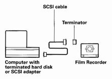
The internal SCSI hard disk or the SCSI host adapter is internally terminated. Therefore, you only need to add one terminator between the cable and the HR 6000 film recorder.
